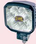
PHARE 6 LED - 18 W 227.- HT Art. 1GA 996 188-001 • 9-33 V - 850 Lm • L112 x 95 mm
